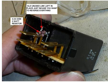
Suitable resistors are available from Radio Shack online Catalog #: 55050377 or NTE part 2WD33 0.33-Ohm for \$1.09 each.
