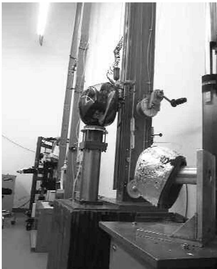
Helmet smackdown —the monorail machine drops a helmet with an instrumented headform inside it from a distance of 6' onto a flat anvil for the DOT standard test. Note that the DOT 6' test corresponds to the 90th percentile of actual accident impacts, unlike Snell's higher impact standards, which Hurt says were chosen simply to be tougher to pass. In fact, he says, in an accident, the harder construction necessary to pass Snell tests can do more damage to a rider's head than the softer DOT-spec helmet, and that a DOT-spec helmet can pass any government required testing in the world.
