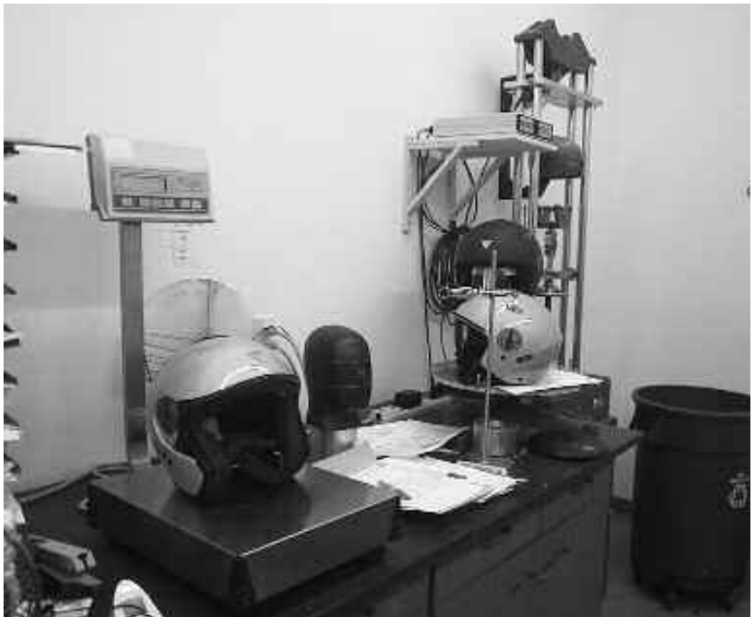
Helmets are carefully weighed and measured as part of the testing procedure. In this photo, the chin strap strength tester and the roll-off test machines are the devices to the right. In the corner is a large pail in which helmets are thoroughly soaked before wet testing. A refrigerator and an oven are also used to duplicate the effects of extremes of ambient temperature on helmet performance.
